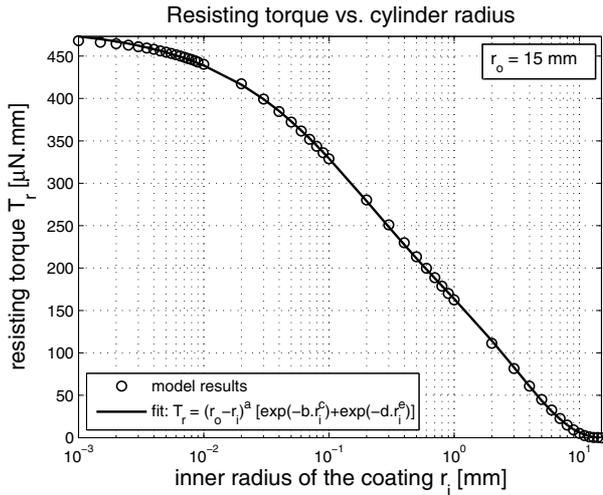
Fig. 7. Variations of the resisting torque  $T_r$  with the inner radius  $r_i$  of the viscoelastic coating, for  $r_o = 15$  mm and  $\Omega = 10$  rps.
