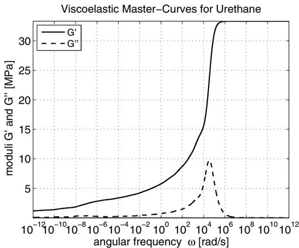
Fig. 3. Frequency-domain master-curves of the Urethane rubber coating.
