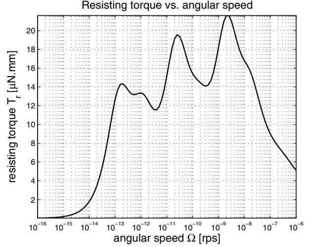
Fig. 5. Variations of the viscoelastic resisting torque with the angular speed.
