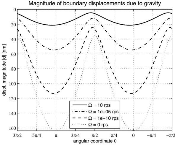
Fig. 4. Variations of the displacement field magnitude over the outer boundary of the viscoelastic coating with the angular coordinate  $\theta$ , for different values of the angular speed  $\Omega$ .
