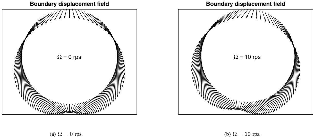
Fig. 2. Quiver plot of the displacement field of the outer boundary of the viscoelastic coating (a) at rest and (b) at an angular speed of  $\Omega = 10$  rps. A purely elastic coating would behave as in (a), regardless of the angular speed.
