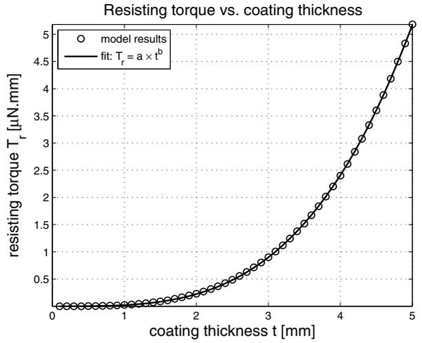
Fig. 6. Variations of the viscoelastic resisting torque with coating thickness, for  $r_i = 10$  mm and  $\Omega = 10$  rps.
