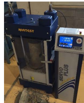
Figure 5 Loading-frame used in compressive strength testing
